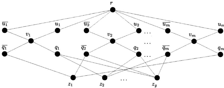
**Fig. 1.** The reduction graph for the  $\langle 3, 1 \rangle$ -edge layout problem
