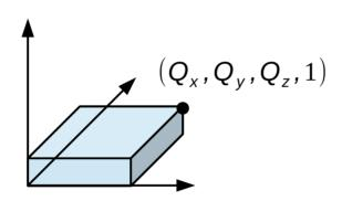
$$Q = \begin{pmatrix} Q_x \\ Q_y \\ Q_z \\ 1 \end{pmatrix} = \begin{pmatrix} S_x & 0 & 0 & 0 \\ 0 & S_y & 0 & 0 \\ 0 & 0 & S_z & 0 \\ 0 & 0 & 0 & 1 \end{pmatrix} \begin{pmatrix} P_x \\ P_y \\ P_z \\ 1 \end{pmatrix} = SP$$
