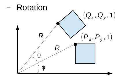
$$Q = \begin{pmatrix} Q_x \\ Q_y \\ 1 \end{pmatrix} = \begin{pmatrix} \cos \theta & -\sin \theta & 0 \\ \sin \theta & \cos \theta & 0 \\ 0 & 0 & 1 \end{pmatrix} \begin{pmatrix} P_x \\ P_y \\ 1 \end{pmatrix} = RP$$
