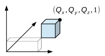
$$Q = \begin{pmatrix} Q_x \\ Q_y \\ Q_z \\ 1 \end{pmatrix} = \begin{pmatrix} 1 & 0 & 0 & T_x \\ 0 & 1 & 0 & T_y \\ 0 & 0 & 1 & T_z \\ 0 & 0 & 0 & 1 \end{pmatrix} \begin{pmatrix} P_x \\ P_y \\ P_z \\ 1 \end{pmatrix} = TP$$
